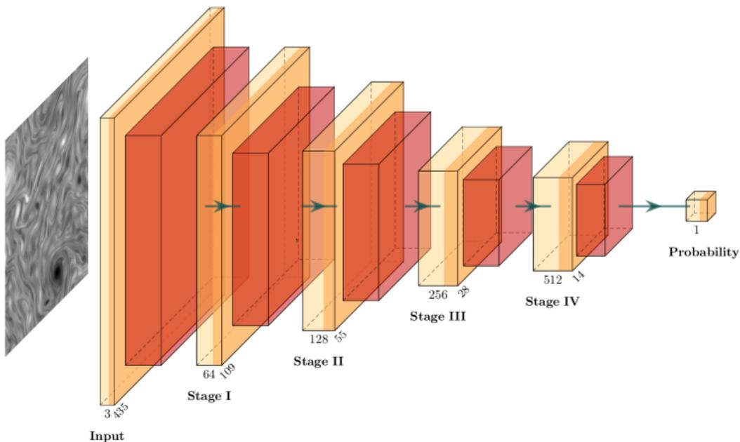
**Figure:** Schematic of the CNN. Each stage represents a set of convolutional layers.
