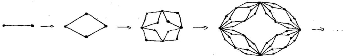
The dots denote lattice sites and the solid lines nearest neighbour bonds. One construction step consists in replacing each bond by a quadrangle. Here we have only performed the first three steps, but the construction can be repeated ad infinitum. On this network we consider the Ising model with Hamiltonian
