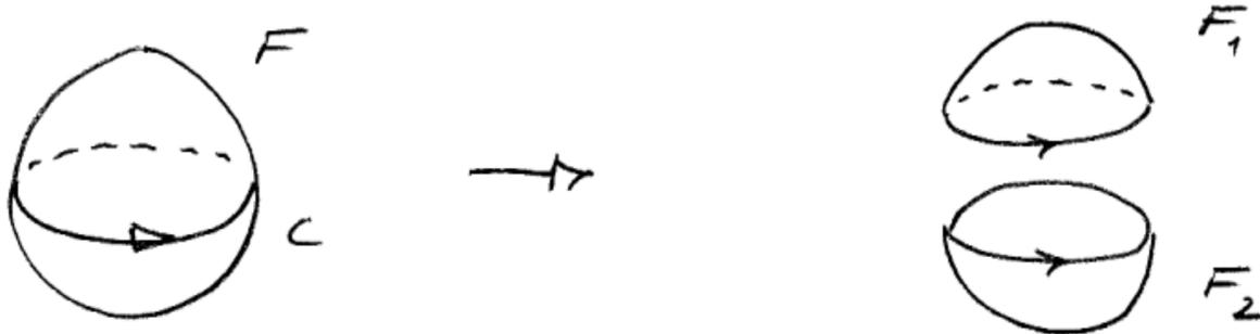
$$\Lambda \int_{F_1} d\vec{f}_1 \cdot \vec{B} = \int_{F_2} d\vec{f}_2 \cdot \vec{B} \quad \text{mit } d\vec{f}_{1,2} = \pm d\vec{f}$$
